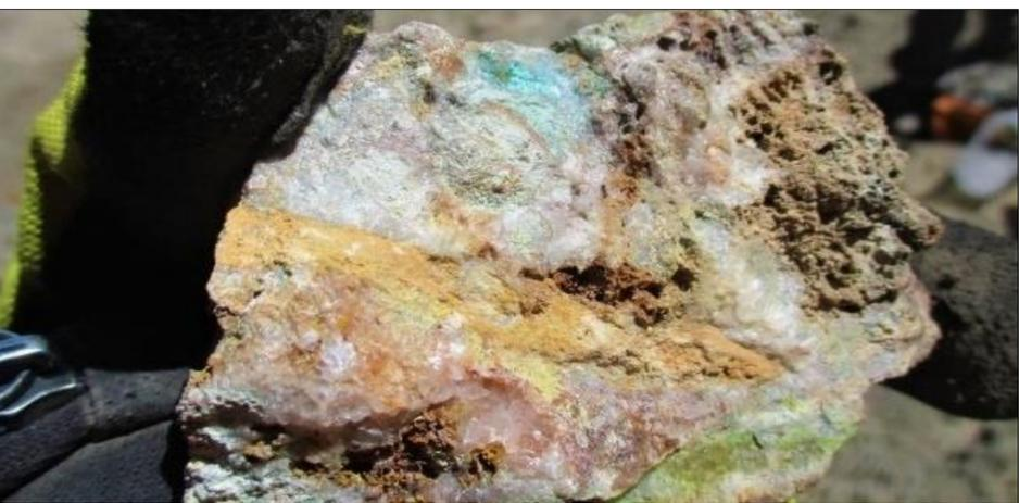
Quartz vein breccia with sulphides. 0.285% Cu, 3,220ppm Mo, 1.02% Pb, 20.3ppm Sb, 292ppm Zn
